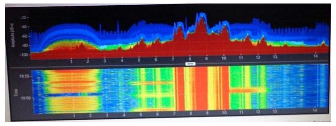
An engineer is troubleshooting non-802.11 interference and observes the shown output. Which interference signature is the most harmful to Wi-Fi?
