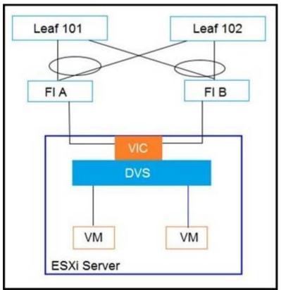
Between Cisco UCS FIs and Cisco ACI leaf switches, CDP is disabled, the LLDP is enabled, and LACP is in Active mode.
