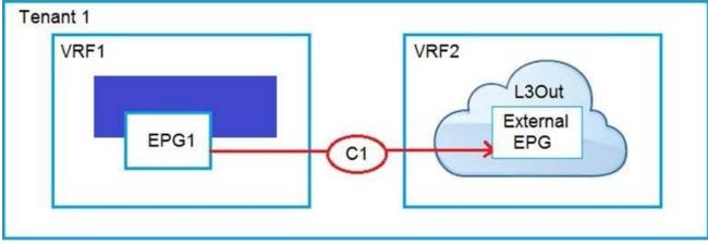
An engineer must have communication between EPG1 in VRF1 and External EPG in VRF2.
