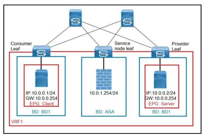
What must be configured in the service graph to redirect HTTP traffic between the EPG client and EPG server to go through the Cisco ASA firewall?
