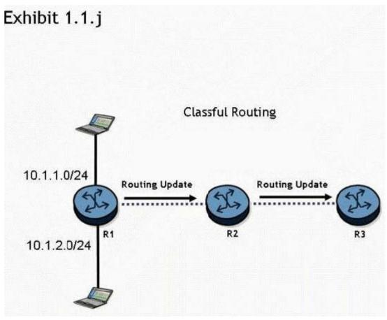
Routers R1 " R2, and R3 are running a classful routing protocol between them. Assuming that router R1 advertises all directly connected networks, how will these networks be represented in router R3's routing table?
