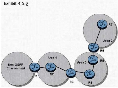
In the topology shown, router R1 is an ASBR configured to export external routes to OSPF. Assuming that there are no stub networks, which of the following statements regarding type 4 LSA generation is true?
