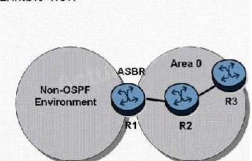
In the topology shown, router R1 is an ASBR configured to export external routes to OSPF. How many type 4 LSAs will be present in the network?
