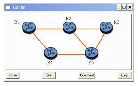
Assuming that LSP R1-R2-R3 requests the default fast reroute configuration, which router becomes a DMP for the detour tunnels?
