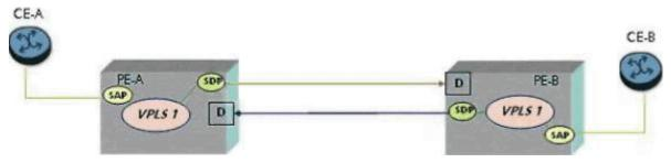
Assume the port on CE-A is sending two tags, a top tag of 100 and a bottom tag of 500. PE-A is configured with a SAP id of 1/1/1:100.\*.
