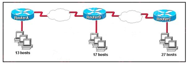
The internetwork is using subnets of the address 192.168.1.0 with a subnet mask of 255.255.255.224. The routing protocol in use is RIP version 1.
