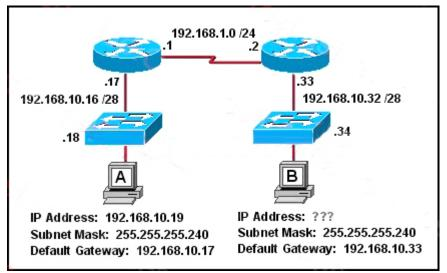
Host B has just been added to the network and must acquire an IP address.
