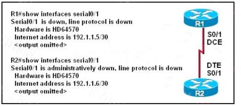
A network technician is unable to ping from R1 to R2. Using the output of the show interfaces serial0/1 command, what should the administrator do to correct the problem?
