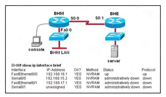
Users on the BHM LAN are unable to access the server attached to the BHE router.
