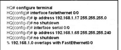
After configuring two interfaces on the HQ router, the network administrator notices an error message. What must be done to fix this error?
