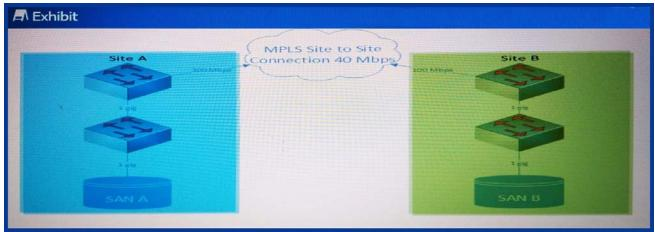
A network engineer is called onsite to troubleshoot replication failure and traffic loss. Whenever replication occurs between SAN A and SAN B, users report traffic loss between sites, and replication ultimately fails due to traffic loss.
