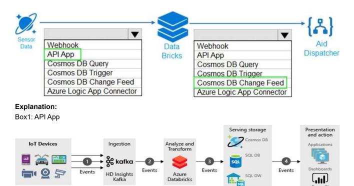
⇒ Events generated from the IoT data sources are sent to the stream ingestion layer through Azure HDInsight Kafka as a stream of messages. HDInsight Kafka stores streams of data in topics for a configurable of time.
