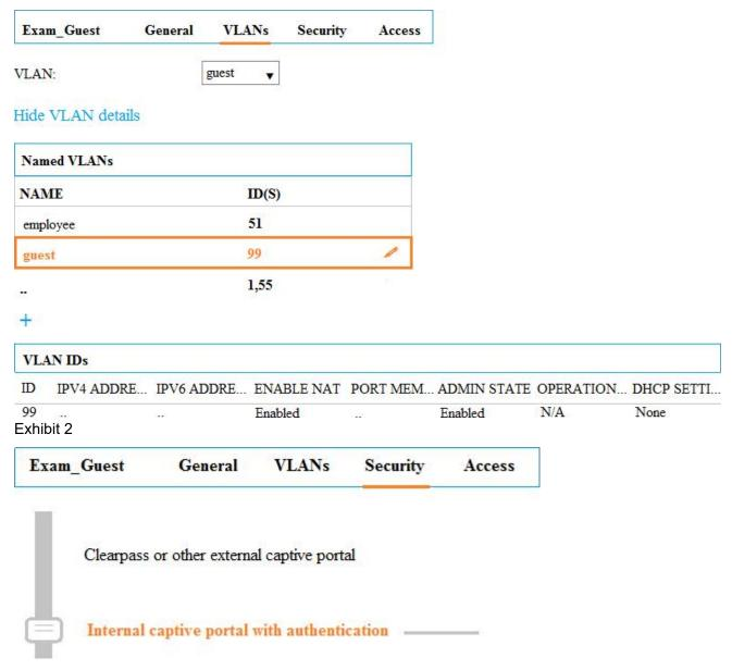
A network administrator configures a guest WLAN on an Aruba Mobility Master (MM)-based solution. The exhibits show some of the settings for this WLAN.
