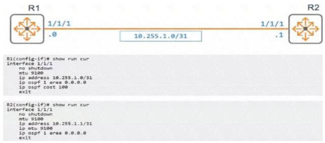
An engineer has applied the above configuration to R1 and R2 However the routers OSPF adjacency never progresses past the "EXSTART-DR" slate as shown below.
