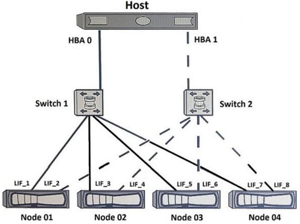
A customer is testing a dual-fabric FC SAN configuration as shown in the exhibit.
