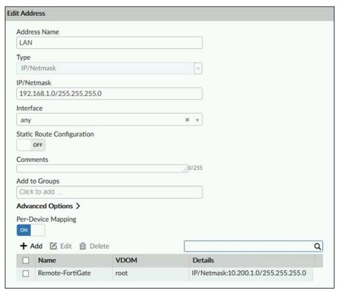
An administrator has created a firewall address object which is used in multiple policy packages for multiple FortiGate devices in an ADOM.
