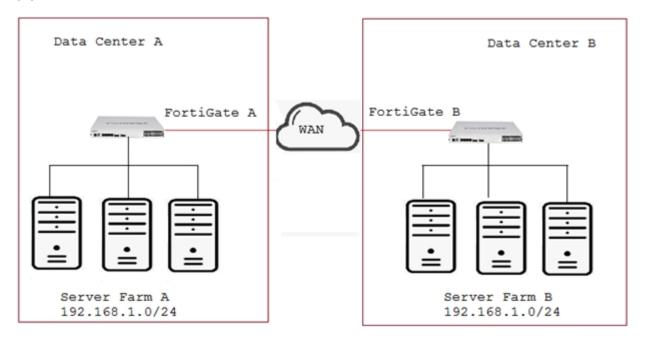
Your company has two data centers (DC) connected using a Layer 3 network. Servers in farm A need to connect to servers in farm B as though they all were in the same Layer 2 segment.
